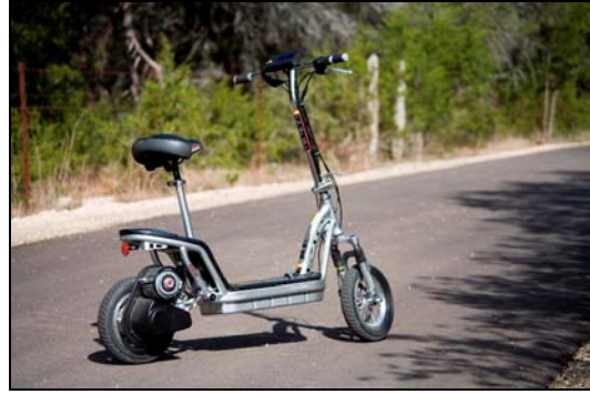
Figure 9: CVP Enabled Currie IZIP 1000 Scooter
